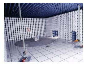
ETS-Lindgren FACT™10 Chambers, for Full Compliance testing, offer semi-anechoic radiated emissions (RE) and fully anechoic radiated immunity (RI) compliance test capability for most international EMC compliance regulations. The chamber's small overall size results from the use of brand hybrid absorber and ferrite tile, which require less volumetric space than traditional absorbers. ETS-Lindgren FACT 10
